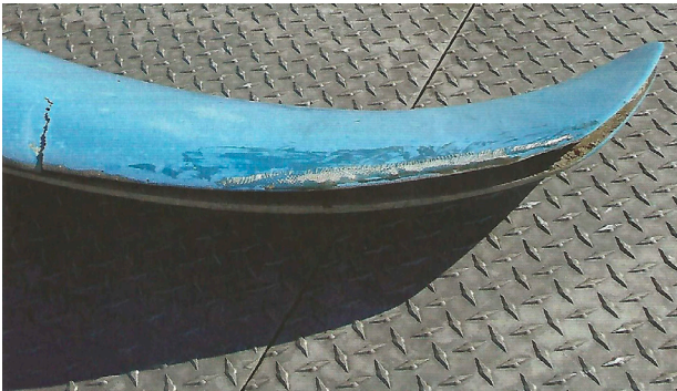
A cracked-up fibreglass impeller
